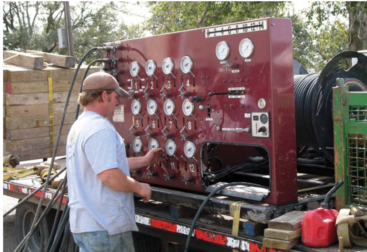
Modern control panel for unified mechanical jacking system.
