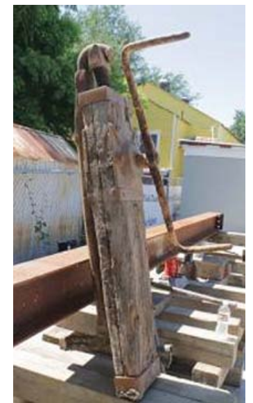
Late-19th-century cotton jack once used by Abry Bros., Inc. to lift buildings.
